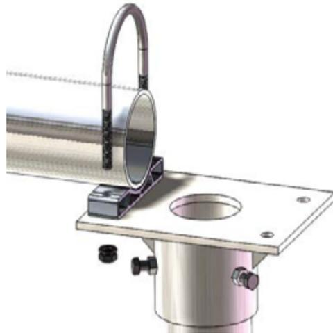
6. Slide the Beam symmetrical onto the Cap. Make sure the marked middle of the Beam is in the middle of the Cap. Place the second Beam Washer under the Beam and mount it as shown in the picture below:
