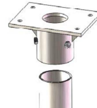
3. Fix the Cap with three Bolt M10x25 to the Pole. Please use a torque wrench (32Nm).
