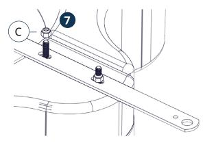
Slide the power cord between the float and screen where two float sections come together before replacing the 3/8" lock nuts.
