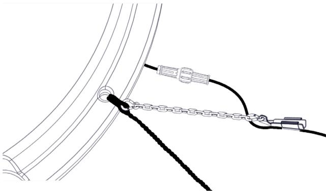
Providing strain relief on the cord helps ensure that its weight and any strain placed on it in the water will not cause the float to tilt or cause damage to the unit.
