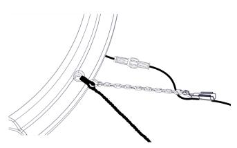
Providing strain relief on the cord helps ensure that its weight and any strain placed on it in the water will not cause the float to tilt or cause damage to the unit.
