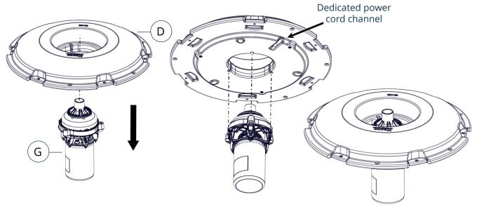
2. Using the 9/16" side of the wrench tool (J) or a socket wrench, secure the float to the unit assembly using the  $3/8 - 16 \times 3$ " hex head screw (A), 3/8" lock washer (B), and  $3/8 \times 1.25$ " fender washer (C), threading into the holes in the baseplate. Repeat for all three holes.
