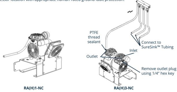
No-cabinet systems arrive assembled. To prepare for installation:
