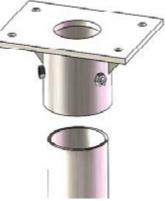
3. Fix the Cap with three Bolt M10x25 to the Pole. Please use a torque wrench (32Nm).
