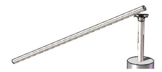
5. Place the Cross Beam Bracket under the Beam, insert the U-bolt (6) into the holes and through the Rack Head, connect M10 washers and lock washers and Nuts. tighten them lightly.
